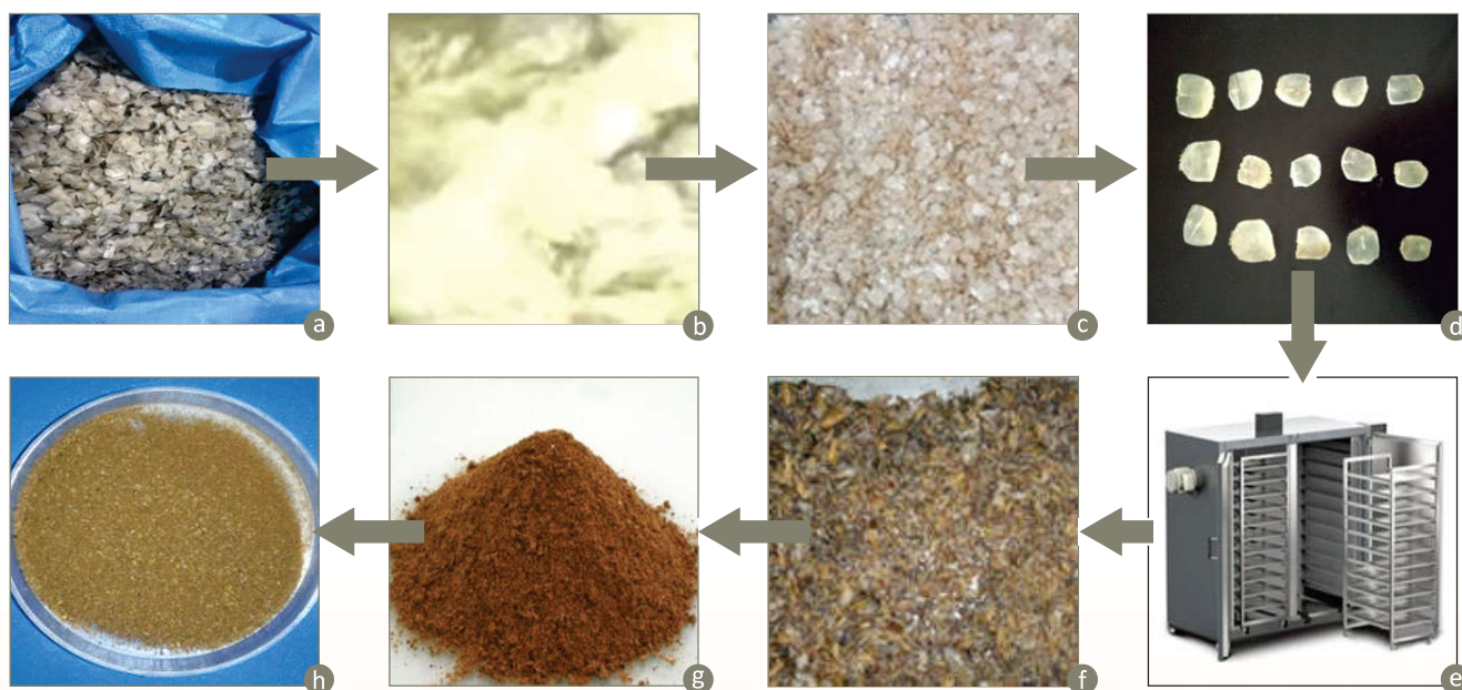
Figure 2: (a) collected scales, (b) soaking, (c) cleaned scales, (d) spread, (e) tray Dryer, cooling, (g) ground powder, (h) fine powder
